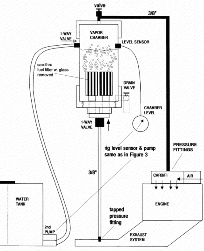
FIGURE 6 OPTIONAL WATER COOLING
